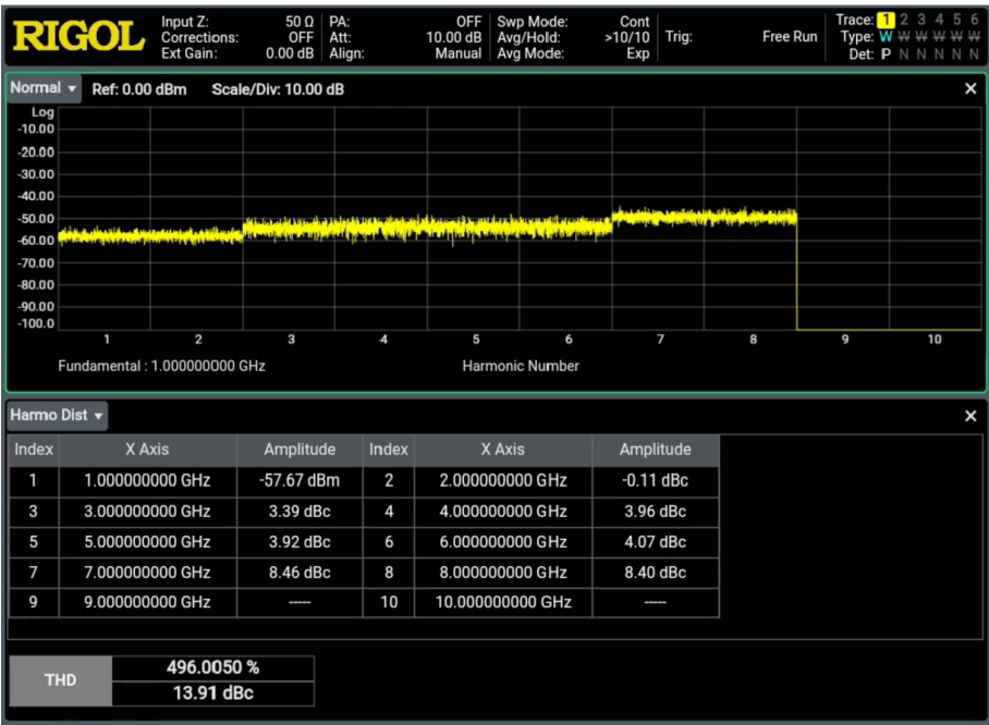
Figure 5.7 Harmonic Distortion Measurement Interface
