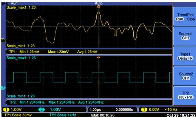
To find intermittent faults the TrendPlot™ function can monitor measurements for long periods of time.
