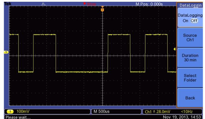
Data logging enables automatic saving of triggered waveforms.
