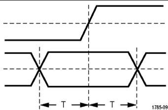
Trigger when a logic data input changes state inside of the setup or hold time relative to a clock edge.
