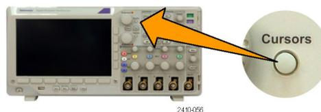
6. Place one cursor on the first peak of the ring using multipurpose knob **a**.
