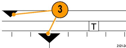
4. The waveform record view shows the trigger location relative to the waveform record. The line color corresponds to the selected waveform color.
