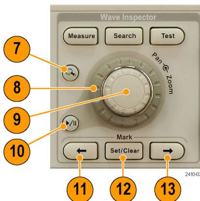
10. **Play-pause** button. Push to start or stop the automatic panning of a waveform. Control the speed and direction with the pan knob.
