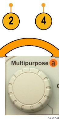
3. Turn multipurpose knob **a** to select the specific measurement. If needed, then turn multipurpose knob **b** to select the channel to measure on.
