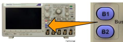
6. Push the **Bus Display** lower-bezel button, push the **Bus and Waveforms** side-bezel button, and push the **ASCII** side-bezel.
