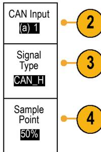
5. Push **Bit Rate** and turn multipurpose knob **a** to select from the list of predefined bit rates.
