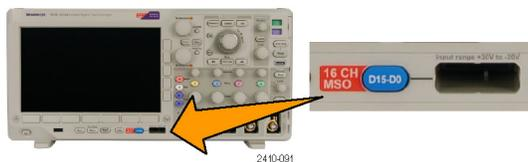
4. Push the **D15-D0 On/Off** lower-bezel button and then push the **Turn On D7-D0** side-bezel to display the digital waveforms. To turn off a channel, use multipurpose knob **a** to select the channel and push the **Display** side-bezel to select Off.
