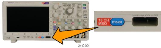
6. Push the lower-bezel **D15 - D0** button to access the D15 - D0 On or Off menu.
