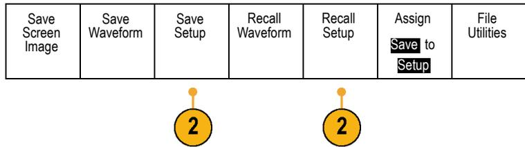
3. From the resulting side-bezel menu, select the location to save the setup to or to recall it from.
