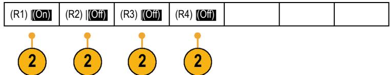
**Removing a reference waveform from the display.** To remove a reference waveform from the display:
