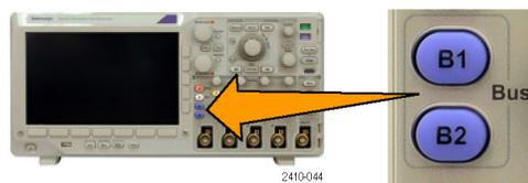
2. Push a lower-bezel **Label** button to create a label, such as for channel 1 or B1.
