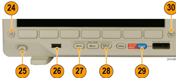
**26. USB 2.0 host port.** Insert a USB cable here to connect peripherals to the oscilloscope, such as a keyboard, a printer, or a flash drive. There is one more USB 2.0 host port on the rear panel.
