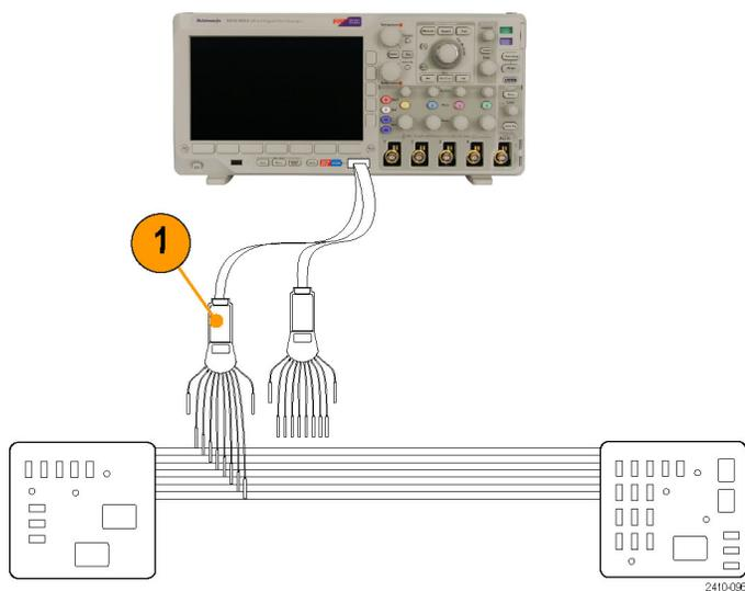
2. Push **Default Setup**. Then push the channel **1** button to remove the waveform from the display.
