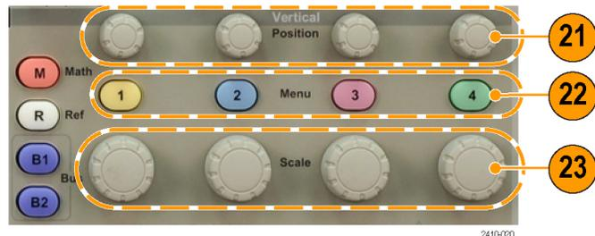
22. **1, 2, 3, 4.** Push to display or remove the corresponding waveform from the display and access the vertical menu.
