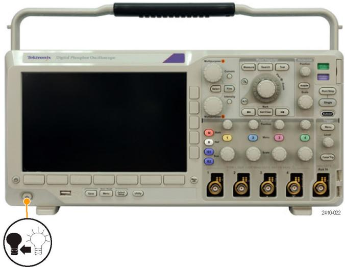
3. Insert the USB flash drive into the front-panel USB port on your oscilloscope.
