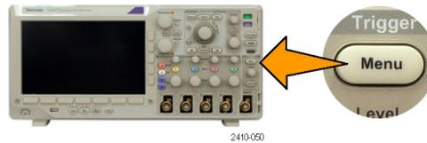
2. Push **Type** to bring up the **Trigger Type** side-bezel menu.
