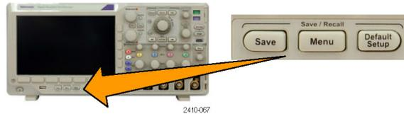
2. Push **Save Waveform** or **Recall Waveform** from the lower-bezel menu.
