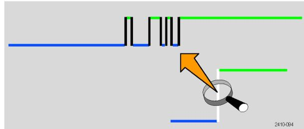
When the oscilloscope is zoomed in so far that there is more than one pixel column per sample, the uncertainty of the edge position is indicated by light gray shading.
