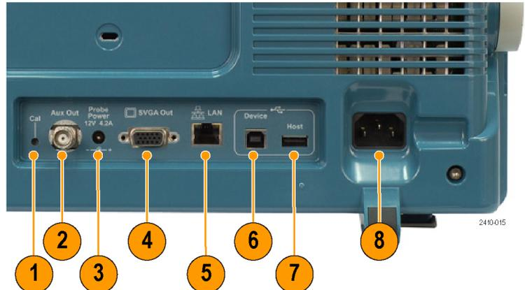
6. **Device.** Use the USB 2.0 High speed device port to control the oscilloscope through USBTMC or GPIB with a TEK-USB-488 Adapter. The USBTMC protocol allows USB devices to communicate using IEEE488 style messages. This lets you run your GPIB software applications on USB hardware. Also, use the USB port to connect a PictBridge-compatible printer to the oscilloscope.
