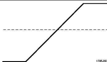
Trigger on a rising or falling edge, as defined by the slope control. Coupling choices are DC, AC, LF Reject, HF Reject, and Noise Reject.
