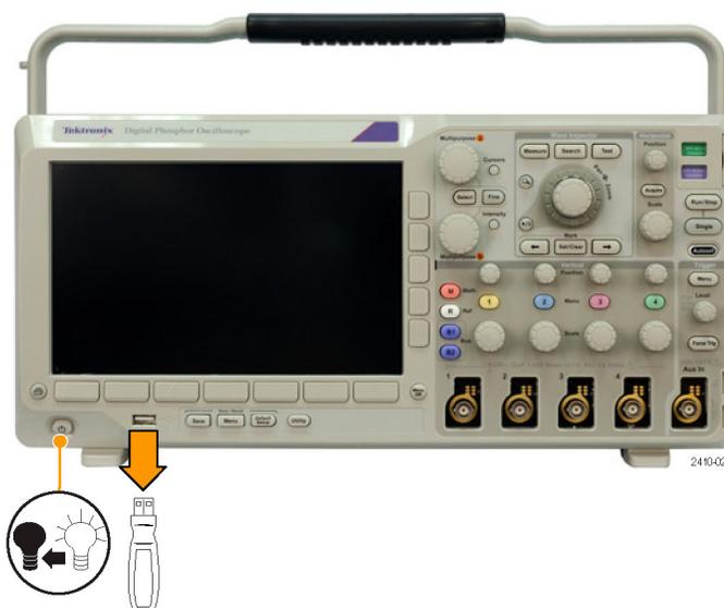
6. Power on the oscilloscope.
