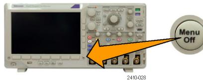
5. Observe that the measurements appear on the screen and update as the signal changes.
