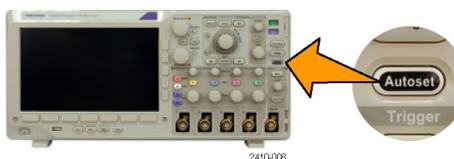
The oscilloscope sets vertical, horizontal, and trigger controls automatically. You can manually adjust any of these controls if you need to optimize the display of the waveform.
