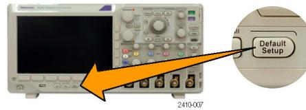
3. Select the input channel by pushing the front-panel buttons.
