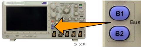
2. Push **Bus**. Turn multipurpose knob **a** to scroll through the list of bus types and select the desired bus: Parallel (MSO3000 Series only), I<sup>2</sup>C, SPI, RS-232, CAN, LIN, or Audio.
