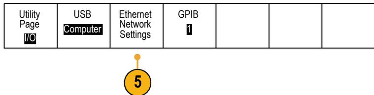
6. On the side-bezel menu, if you are on a DHCP Ethernet network and using dynamic addressing, set DHCP to **On**. If you are using static addressing, set it to **Off**.
