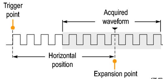
1. Adjust the position (delay) time by rotating the **Horizontal Position** knob.
