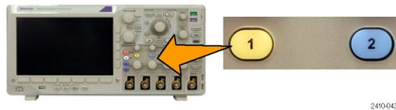
Connect the digital probe and select the input channel. (See page 63, *Setting Up Digital Channels*.)
