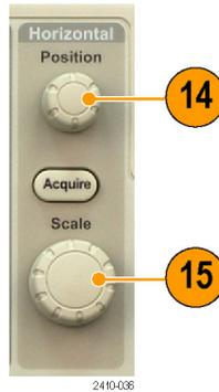
15. **Horizontal Scale.** Turn to adjust the horizontal scale (time/division).
