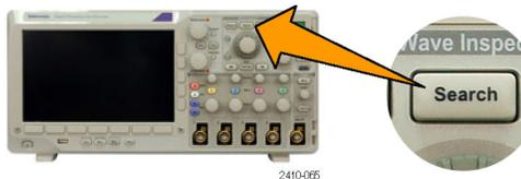
10. Push **Search Type**. Use the multipurpose knob **a** to select **Bus** and then push **Data**. Use the multipurpose knobs **a** and **b** to define the data value.
