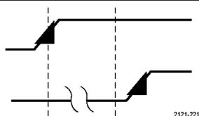
Combine an edge A Event (Main) trigger with the B Event (Delayed) trigger to capture more complex signals. (See page 78, *Using Sequence Trigger, A (Main) and B (Delayed).*)
