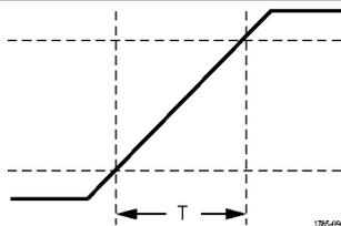
Trigger on rise and fall times. Trigger on pulse edges that traverse between two thresholds at faster or slower rates than the specified time. Specify pulse edges as positive, negative, or either.
