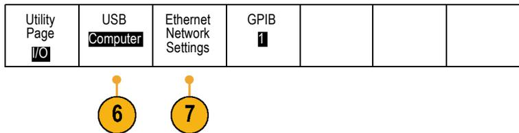
Check **USB** on the lower-bezel menu to be sure that USB is enabled. If it is not enabled, push **USB**. Then push **Connect to Computer** on the side-bezel menu.
