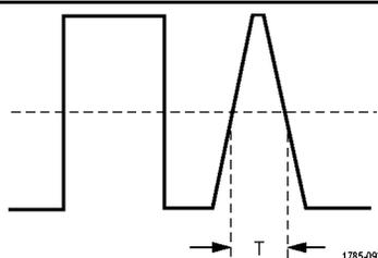
Trigger on pulses that are less than, greater than, equal to, or not equal to a specified time. You can trigger on positive or negative pulses. Pulse width triggers are primarily used on digital signals.
