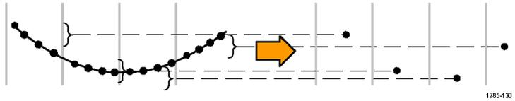
**Envelope** mode finds the highest and lowest record points over all acquisitions. Envelope uses Peak Detect for each individual acquisition.
