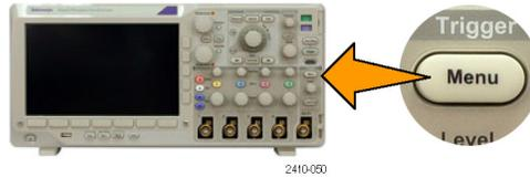
6. Push **Type** to select **Bus**. Enter trigger parameters in the resulting screen menus.
