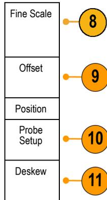
9. Select **Offset** to enable multipurpose knob **a** to make vertical offset adjustments.
