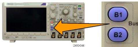
2. Turn multipurpose knob **a** to adjust the vertical position of the selected bus.
