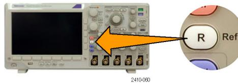
2. Push the **R1, R2, R3, or R4** lower-bezel button to remove the reference waveform from the display.
