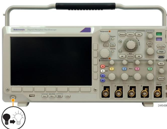
5. Power off the oscilloscope and remove the USB flash drive.
