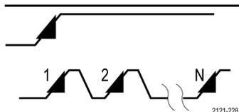
**Events.** After the A Event occurs, the trigger system looks for a specified number of B Events before triggering and displaying the waveform.
