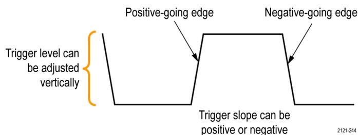
The oscilloscope provides a long horizontal bar or bars across the graticule to temporarily show the trigger level.
