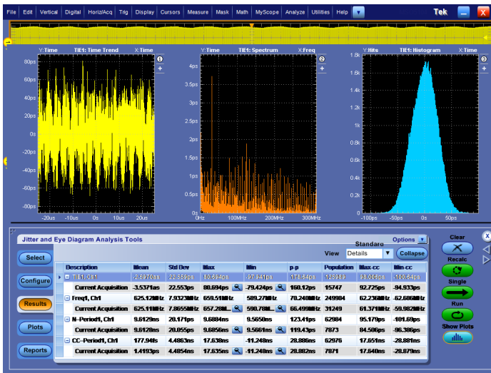
Jitter analysis - TIE jitter/timing analysis of 622 Mb/s signal
