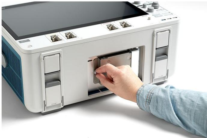
When the SSD is present, the instrument boots in an open Windows 10 configuration, so you can minimize the oscilloscope application and access a Windows desktop where you can install and run additional applications on the oscilloscope. Or you can connect additional monitors and extend your desktop.
