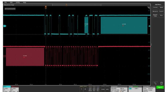
Multiple channel triggering. Visual Trigger areas can be associated with events spanning multiple channels such as packets transmitted on two bus signals simultaneously.
