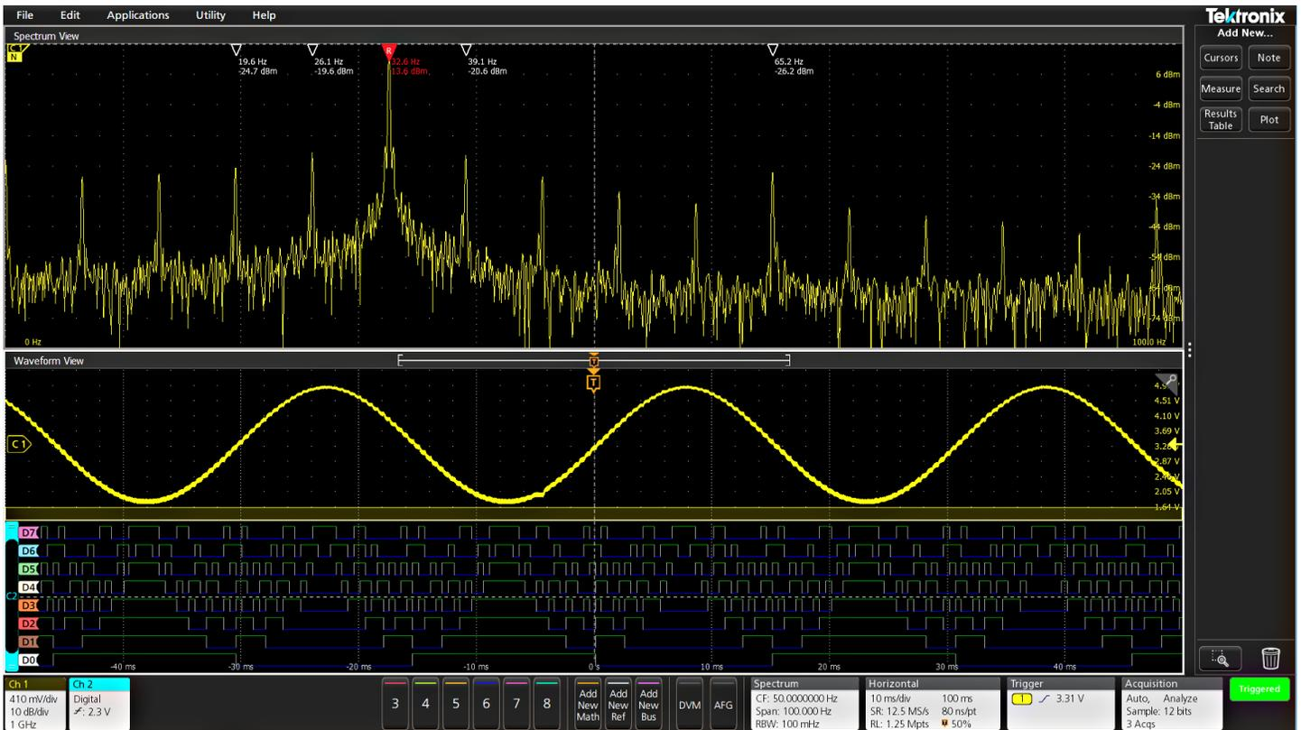
Beyond just analog and digital, FlexChannel inputs include Spectrum View. This Tektronix-patented technology enables you to simultaneously view both analog and spectral views of your signal with independent controls in each domain. For the first time ever, oscilloscope-based frequency-domain analysis is as easy as using a spectrum analyzer while retaining the ability to correlate frequency-domain activity with other time-domain phenomena.
