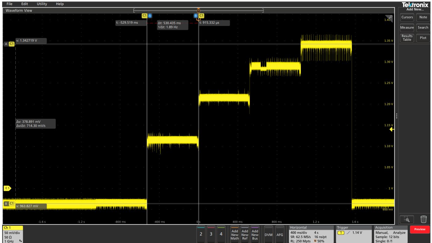
Figure 11. Example of a device that is scaling the input voltage needed as the frequency is increased. The \sim 2 Hz frequency component between steps will be missed with many AC coupling filters
