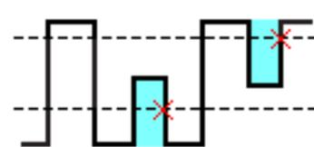
A runt pulse is a pulse that crosses one threshold but fails to cross a second threshold before recrossing the first. Therefore, a runt trigger needs two thresholds to define the two levels that a signal must pass through to be considered a valid (nonrunt) signal.
