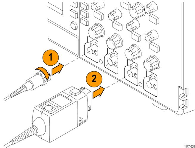
2. Tektronix Versatile Probe Interface (TekVPI®): Push the probe base into the channel connector until the probe base connector clicks. To remove, push and hold the button on the probe base and pull the probe from the connector. TekVPI® probes automatically set the oscilloscope probe parameters such as type (voltage, current) and attenuation (10X, 1X, X10, and so on).
