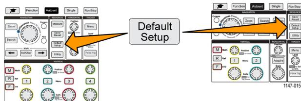
2. If you change your mind, push **Undo Default Setup** side-menu button to return the oscilloscope to the settings present before you pushed **Default Setup**. You must push this button before doing any other action.
