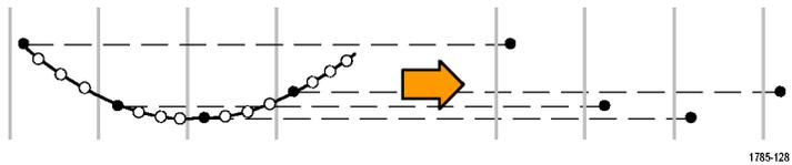
**Peak Detect** mode uses the highest and lowest of all the samples contained in two consecutive acquisition intervals. Use this mode to help detect short rapid transitions in a waveform. Peak Detect is not available at faster time per division settings.
