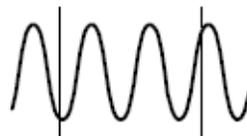
Time readouts are relative to the trigger point (which is 0 s). For example, cursors to the left of the trigger are minus time values.
