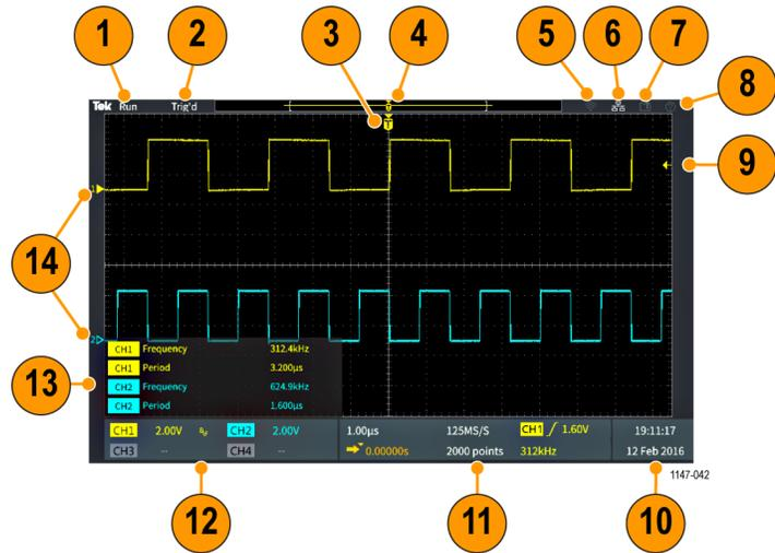
1. The acquisition status shows when an acquisition is running, stopped, or when acquisition preview is in effect. The acquisition modes are:
