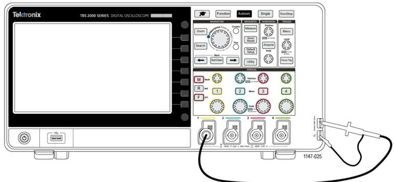
5. Push **Default Setup**. Default Setup returns the oscilloscope settings to factory default values. (See page 111, *The default oscilloscope settings (Default Setup)*.)
