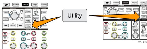
2. Push **Set Date & Time** side-menu button. The oscilloscope shows the **Set Date & Time** menu.
