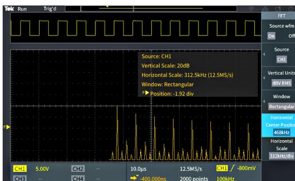
8. Push the **Horizontal Scale** side-menu button and use the **Multipurpose** knob to set the horizontal scale (frequency per major graticule division) value. Use this to expand or contract the FFT waveform to show more or less detail. The FFT waveform expands around the center cursor.
