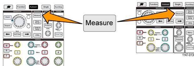
3. Push the side-menu button of the channel for which to show the measurement snapshot. You can only take a snapshot of one channel at a time.
