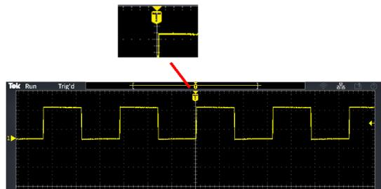
4. The waveform record view shows the trigger location relative to the entire waveform record. The line color corresponds to the selected waveform color. The area in brackets is the part of the waveform record that is displayed on the screen.
