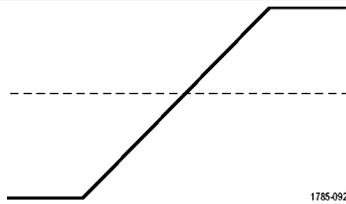
Edge triggers are the simplest and most commonly used trigger type. An edge trigger event occurs when the trigger source passes through a specified voltage threshold (trigger level) when the signal is transitioning in the specified slope (rising or falling).
