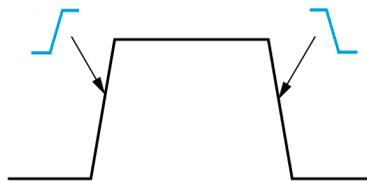
The trigger threshold **Level** (or just level) is the signal amplitude value on a slope that must occur for the oscilloscope to trigger on a signal.
