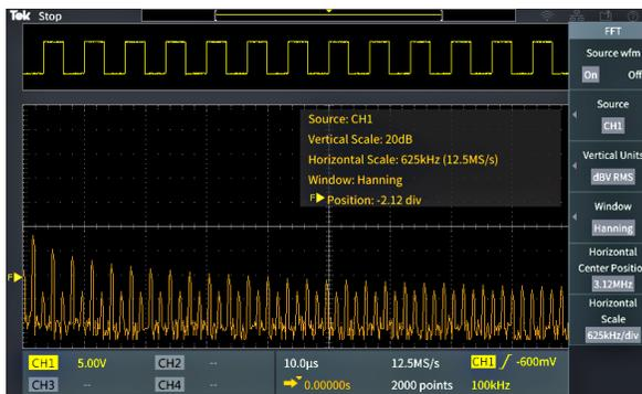
3. Push **Source wfm** side-menu button to toggle the display of the source waveform (at the top of the screen) **On** or **Off**.
