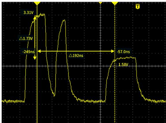
Cursor readouts appear next to the cursors. The readouts show the signal values at the current cursor positions. The readouts also show the difference (delta, marked with a  $\Delta$  symbol) between the cursor measurements. The oscilloscope always shows the readouts when the cursors are turned on.
