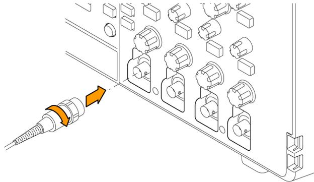
4. Connect the probe tip and ground lead to the **PROBE COMP** connectors on the oscilloscope front panel. The probe tip connects to the 5 V connector, and the ground clip connects to the ground connector.
