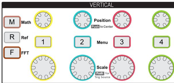
The Vertical controls set the vertical settings (position and scale) for each channel, and enable turning on or off individual waveforms.
