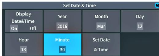
7. When you have finished making all date and time changes, turn the **Multipurpose** knob to select **Set Date & Time**, then click the knob to enter the date/time settings into the oscilloscope.
