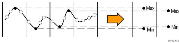
**Hi Res** mode oversamples lower-frequency signals and calculates the average of all the samples for each acquisition interval. Use Hi Res mode to provide higher-resolution (16-bit) sample points for lower-frequency waveforms.
