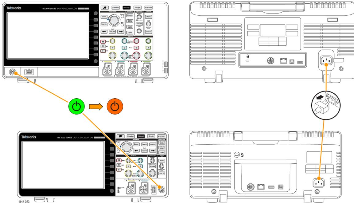
**NOTE.** The current instrument settings are stored in nonvolatile memory when you power off the oscilloscope. The oscilloscope restores the settings when you power on.
