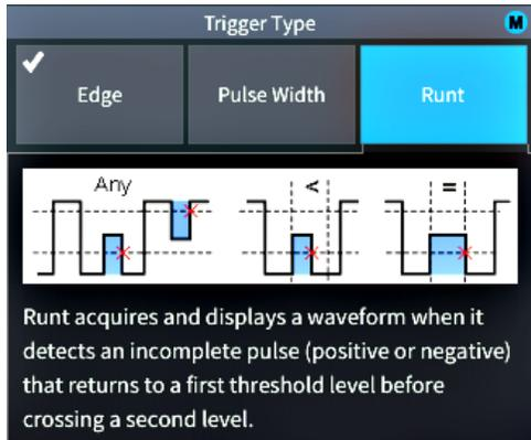
You can enable **Help Everywhere** content for all supported settings, or enable it for specific function groups, such as **Trigger** controls, **Vertical** controls, and so on.
