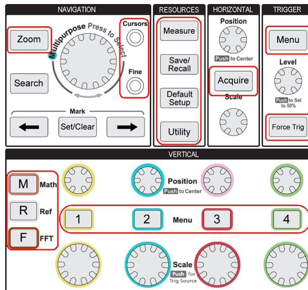
The oscilloscope opens the side menu list for that button on the right side of the screen.
