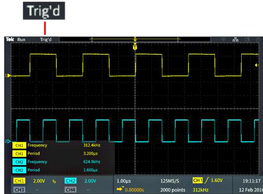
3. The trigger position icon (T) shows where the trigger occurred in the waveform record.
