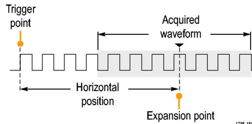
3. With **Delay** set to **On**, the trigger point is disconnected from the expansion point. Turn the **Horizontal Position** knob to move the trigger point away from the expansion point (center graticule). The amount of delay is shown in the Horizontal Status area at the bottom-center of the graticule, referenced to 0 s (center graticule).
