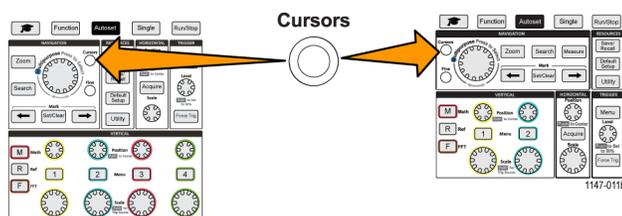
The color of the cursors indicates the channel on which they are taking measurements.
