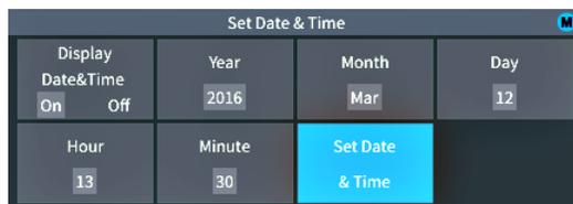
8. To turn off displaying the date and time, select **Display Date & Time** and click the **Multipurpose** knob to toggle **On** or **Off**.
