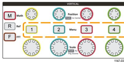
2. Push the **Invert** side-menu button to toggle between **Off** for normal operation and **On** to invert the polarity of the signal in the preamplifier.
