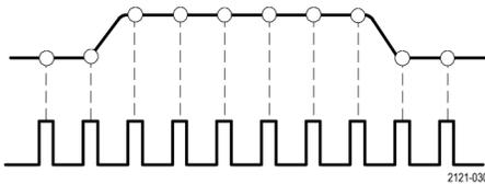
TBS2000 Series oscilloscopes use real-time sampling. In real-time sampling, the oscilloscope samples and digitizes all of the sampled points at one time, in sequence, stores the sampled data in memory, and then repeats the sampling and storage process.
