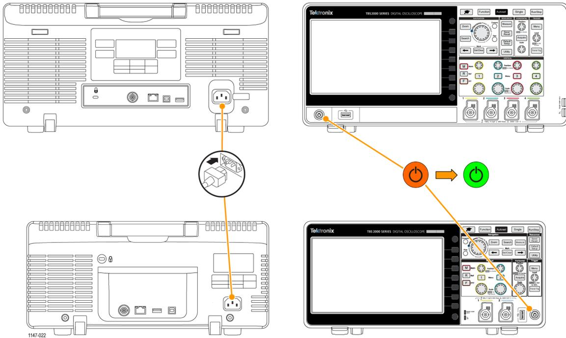
To power off the oscilloscope and remove the power cord:
