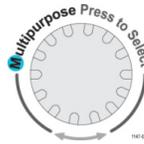
The turn arrow indicator, located below the knob, turns green when you can use the knob to make selections or enter values in a menu or dialog box.
