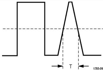
You can trigger on pulses that are less than, greater than, equal to, or not equal to a specified time period. You can trigger on positive or negative pulses.
