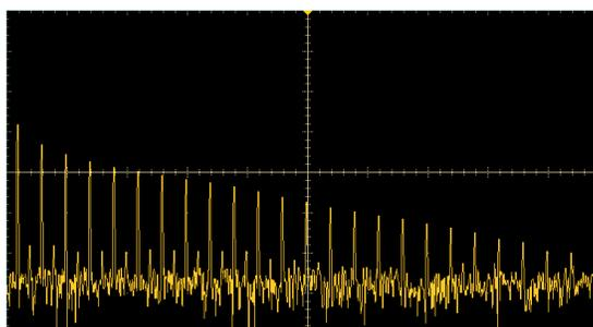
Use the **Linear RMS** vertical scale to see an overall view of how all frequencies levels compare to each other.
