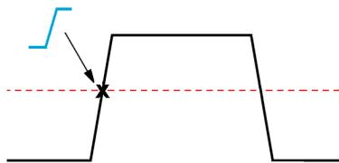
A runt trigger needs two thresholds to define the two levels that a signal must pass through to be considered a valid (nonrunt) signal.
