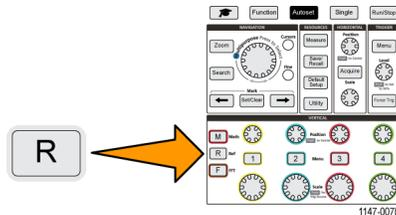
2. Push the **Ref1** or **Ref2** side-menu button to toggle displaying that waveform **On** or **Off**.
