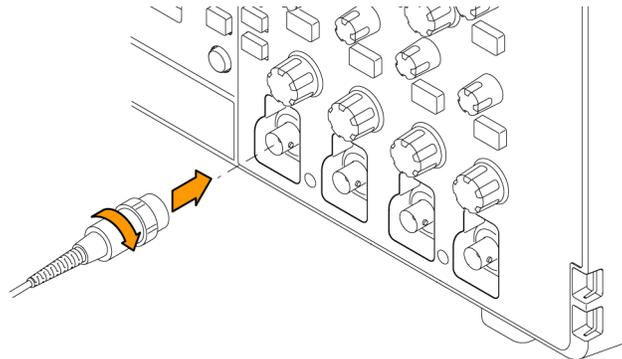
3. Connect the probe tip and ground lead to the **PROBE COMP** connectors on the oscilloscope. The probe tip connects to the 5 V connector, and the ground clip connects to the ground connector.
