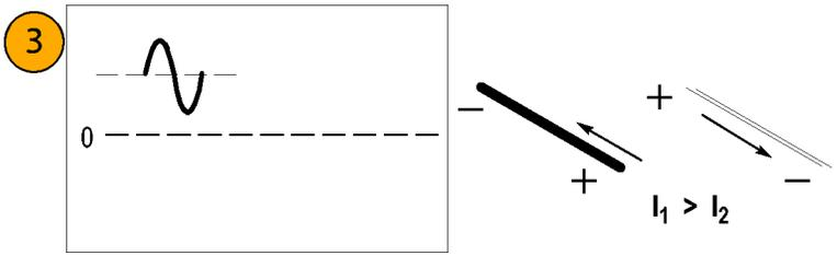
4. To adjust for a current null, adjust the current in one of the conductors until the displayed measurement is zero.
