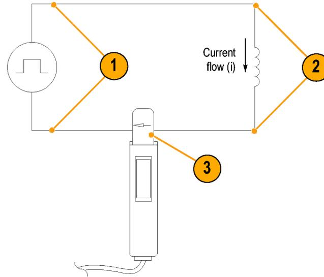
4. Measure the current ramp. The inductance is effectively defined by the slope of the current ramp shown here.
