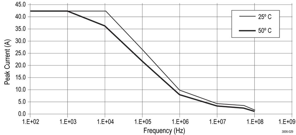
Figure 1: Frequency derating (peak current versus frequency)
