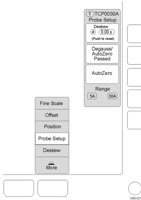
**Deskew.** To deskew the TCP0030A probe to other probes, select this function and connect the probes to the optional deskew fixture. (See page 43, *Deskew/Calibration Fixture*.)
