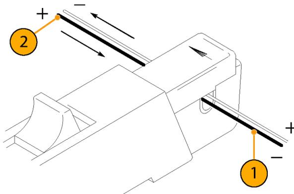
**NOTE.** Adding a second conductor to the probe increases the insertion impedance and reduces the upper bandwidth limit of the probe. Winding multiple turns further increases the insertion impedance, further reducing the upper bandwidth limit.
