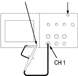
1. Push the **CH 1 MENU ▶ Probe ▶ Voltage ▶ Attenuation** option and select **10X**. Set the switch to 10X on the P2220 probe and connect the probe to channel 1 on the oscilloscope. If you use the probe hook-tip, ensure a proper connection by firmly inserting the tip onto the probe.
