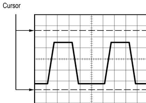
**Cursors** This method allows you to take measurements by moving the cursors, which always appear in pairs, and reading their numeric values from the display readouts. There are two types of cursors: Amplitude and Time.
