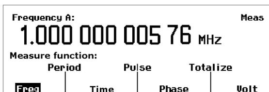
Typical measurements include frequency, period, time, pulse, phase, totalize (FCA3100 Series only), and volts. The measurement menu content depends on the instrument model and configuration.
