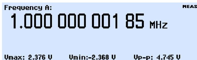
With three input channels, you can measure the relationship between different signals. For example, you can measure the phase relationship between the input and output signals of your device. You can read other critical parameters simultaneously, such as the test frequency of the signal and the voltage ratio (in dB), in one glance with the multi-parameter display.
