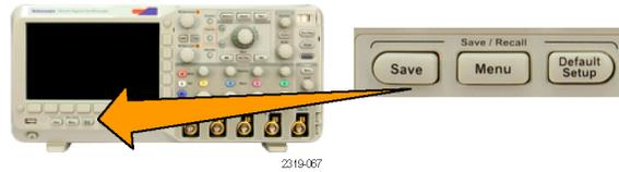
2. Push **Save Screen Image, Save Waveform, or Save Setup**.
