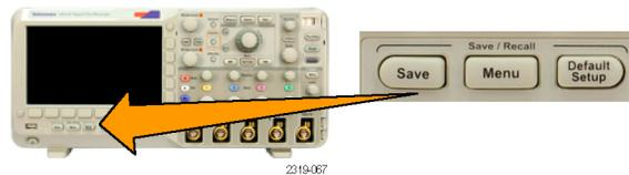
2. Push **Save Setup** or **Recall Setup** from the lower-bezel menu.
