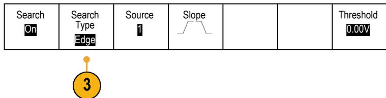
Turn multipurpose knob **a** to select the search type: Edge, Pulse Width, Runt, Logic, Setup & Hold, Rise/Fall Time, or Bus.
