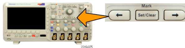
3. Investigate your waveform by moving from search mark to search mark. Use the next (→) or previous (←) arrow button to jump from one marked location to another, without adjusting any other controls.
