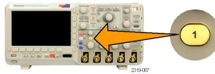
Connect the digital probe and select the input channel. (See page 59, *Setting Up Digital Channels (MSO2000B Series Only).*)
