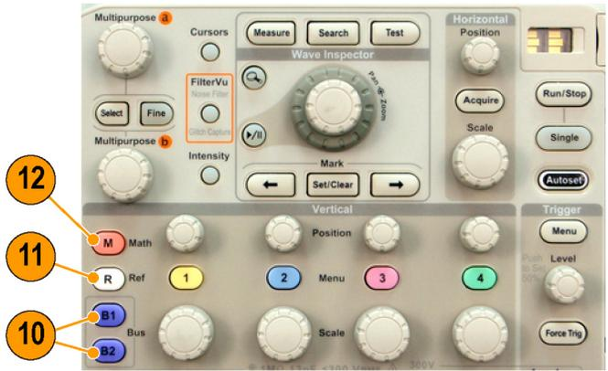
11. **R**. Push to manage reference waveforms, including the display or removal of each reference waveform from the display.
