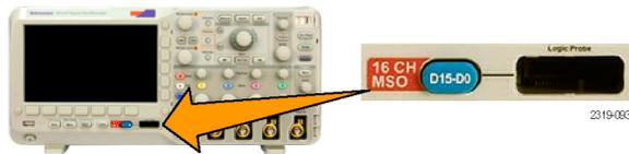
6. Push the lower-bezel **D15 - D0** button to access the D15 - D0 On or Off menu.
