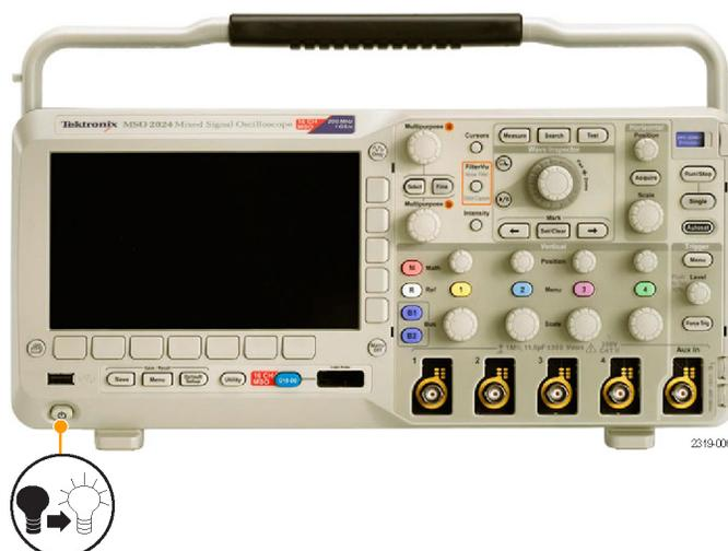
3. Connect the TPP0200/TPP0100 probe tip and reference lead to the **PROBE COMP** connectors on the oscilloscope.
