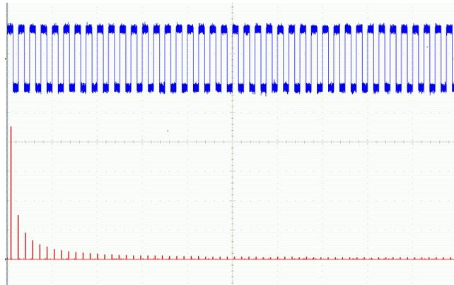
3. Push the side-bezel menu **FFT Source** button and turn multipurpose knob **a** to set the source to channel **1**, **2**, **3**, or to **4**.
