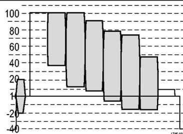
Trigger on specified fields or lines of a composite video signal. Only composite signal formats are supported.
