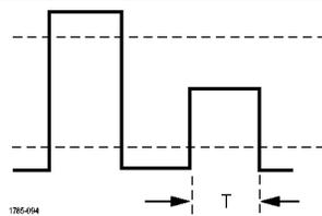
Trigger on a pulse amplitude that crosses one threshold but fails to cross a second threshold before recrossing the first. You can detect positive or negative (or either) runts, or only those wider than, less than, greater than, equal to, or not equal to a specified width. Runt triggers are primarily used on digital signals.
