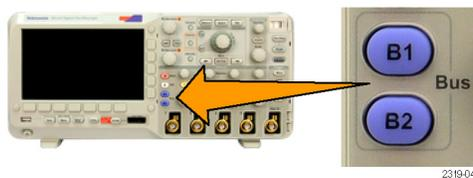
2. Push a lower-bezel button to create a label, such as for channel 1 or B1.
