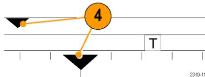
5. The waveform record view shows the trigger location relative to the waveform record. The line color corresponds to the selected waveform color.
