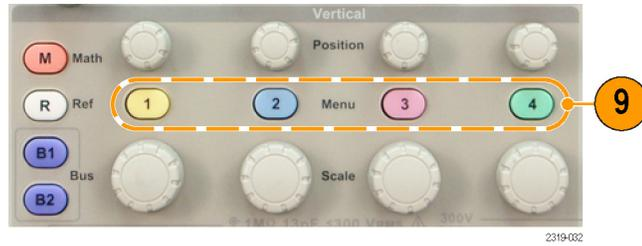
10. **B1** or **B2**. Push to define and display a serial bus if you have the appropriate module application keys. The DPO2AUTO module supports CAN and LIN buses. The DPO2EMBD module supports I<sup>2</sup>C and SPI. The DPO2COMP module supports RS-232, RS-422, RS-485, and UART buses. Parallel bus support is available on MSO2000B products.
