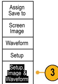
4. From now on, when you push **Save** the oscilloscope creates three files: setup, screen image, and waveform.
