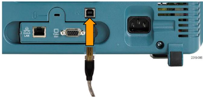
**NOTE.** The oscilloscope recognizes the printer only when the printer is powered on.
