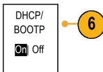
7. Push **Change Instrument Settings**. If you are using DHCP, note the Ethernet address and instrument name. If you are using Static addressing, enter the Ethernet address you will be using.
