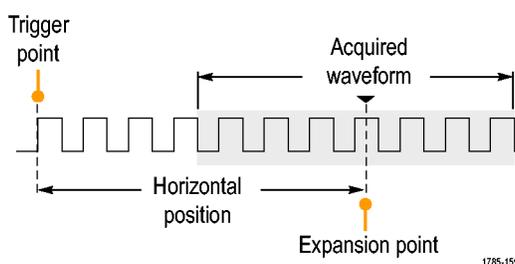
1. Adjust the position (delay) time by rotating the **Horizontal Position** knob.
