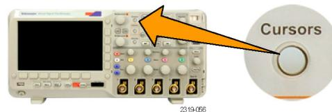
6. Turn multipurpose knobs **a** and **b** to move the pair of horizontal cursors.
