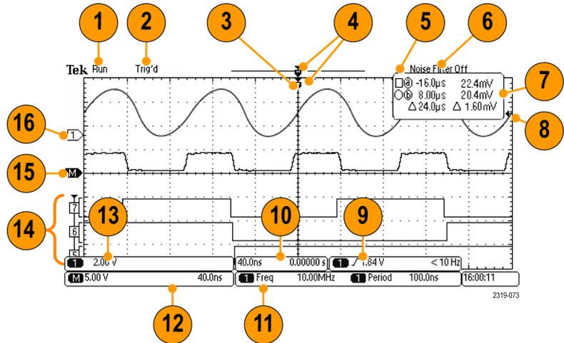
1. The acquisition readout shows when an acquisition is running, stopped, or when acquisition preview is in effect. Icons are:
