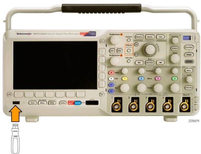
4. Power on the oscilloscope. The oscilloscope automatically recognizes and installs the replacement firmware.
