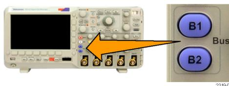
2. Push Trigger **Menu** and enter trigger parameters. (See page 67, *Choosing a Trigger Type*.)
