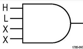
Trigger when all channels transition to the specified state. Use multipurpose knob **a** to select a channel. Push the appropriate side-bezel button to set that channel's state to **High (H)**, **Low (L)**, or **Don't Care (X)**.
