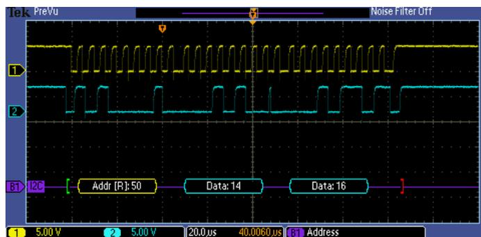
Figure 14: Triggering on a specific data packet going across an I<sup>2</sup>C bus. The yellow waveform is clock and the blue waveform is data. A bus waveform provides decoded packet content including Start, Address, Read/Write, Data, and Stop.
