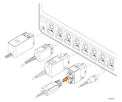
Figure 2: Connecting probes to the MSO54, MSO56, MSO58, MSO54B, MSO56B, or MSO58
