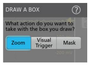
Tap the Draw-A-Box **Zoom icon** button at the up right of the **Results Bar**, then touch and drag in the Waveform view to draw a box on the area of interest. The Zoom mode stays enabled so that you can draw boxes to zoom in different areas of the Zoom Overview, or draw boxes to further zoom in on the same area.
