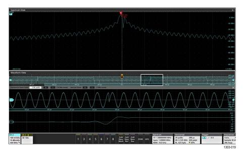
This trace can help characterize phase modulation and phase drift. Changes in phase are not visible in the spectrum trace, and can be difficult to locate in the time-domain signal.
