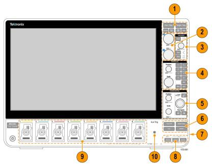
Figure 8: 5 Series B MSO controls
