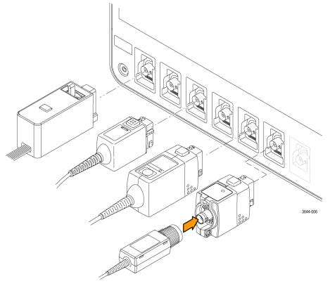
Figure 1: Connecting probes to the MSO44 or MSO46
