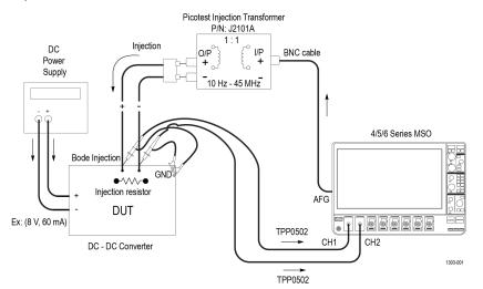
Note: To perform BODE measurement, inject stimulus signal from AFG over a band of frequencies to the control loop feedback path of the power convertor. To facilitate the signal injection, a small resistor needs to be inserted in the feedback loop. The injection resistor value should be of < 10 Ohms (recommended value is around 5 Ohms).
