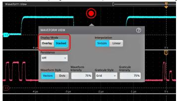
2. Tap the buttons in the Display Mode to toggle between Overlay and Stacked modes.
