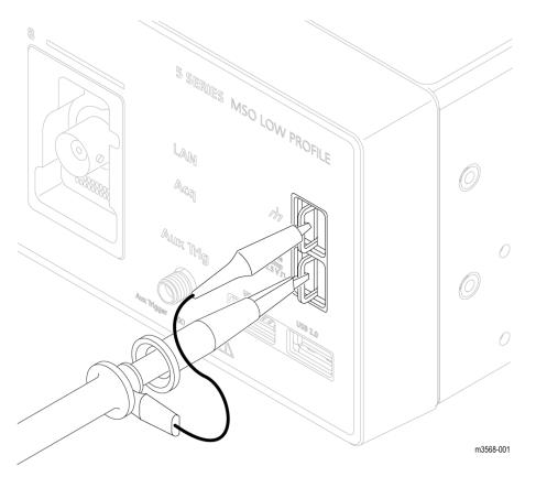
The Probe Compensation connections provide a ground connector and 1 kHz square wave source for adjusting the high-frequency response of a passive probe (probe compensation). The oscilloscope uses this signal to automatically compensate supported probes. See *Compensate the TPP Series probes* on page 80.
