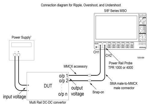
**Connection setup for Digital Power Management (DPM) measurements**
