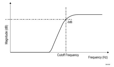
HPF can be used to remove DC and low-frequency components. Both LPF and HPF are commonly used in HSS (High Speed Serial) and data communication applications.
