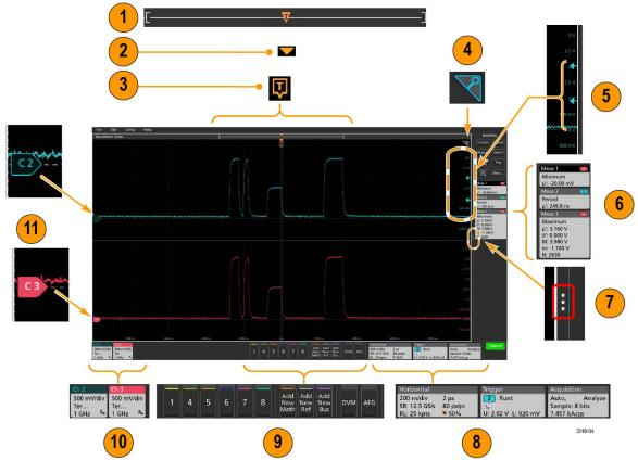
1. The Waveform Record View is a graphical high-level view of the overall waveform record length, how much of the record is on the screen (shown in brackets), the location of key time events including the trigger event, and the current position of waveforms cursors.
