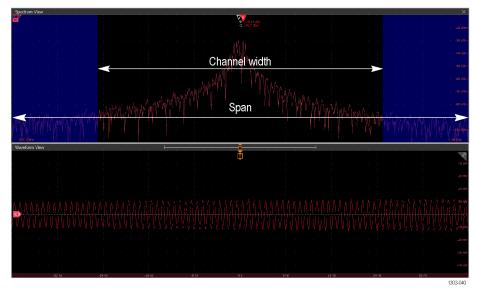
Figure 32: The image shows the channel width for a given Channel Power measurement.
