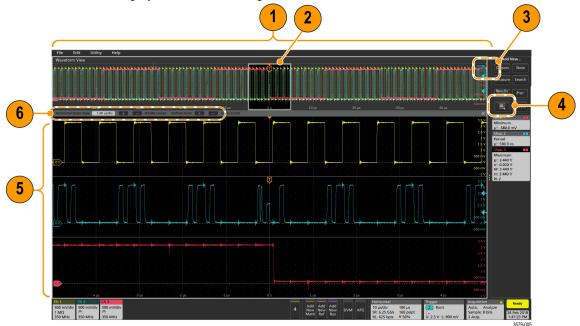
1. The Zoom Overview shows the entire waveform record. All waveforms are shown in Overlay mode in the Zoom Overview area.
