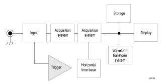
Trigger helps you to capture meaningful waveforms to display on screen. This instrument has simple edge triggers as well as a variety of advanced triggers.
