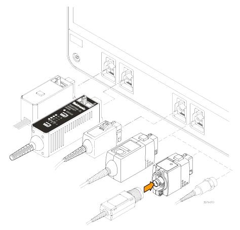
Figure 4: Connecting probes to the MSO6B
