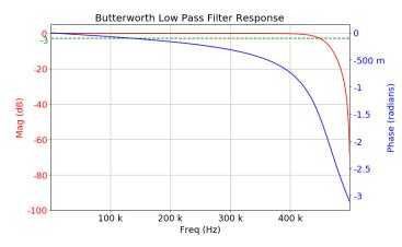
As the filter order is increased, the passband and stop-band performance improve, with the transition from passband to stop-band becoming sharper. The Butterworth method is best suited for design problems that focus on controlling passband and stop-band ripple.
