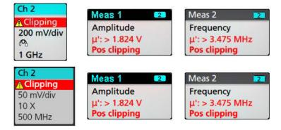
To close the clipping message, change the vertical scale to show the entire waveform, disconnect the probe tip from the excessive voltage source, and check that you are probing the correct signal using the correct probe.
