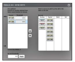
The bus waveform updates as you make changes on the configuration menu. Tap the + symbol next to the waveform handle to turn on and off showing the signals associated with the bus waveform.
