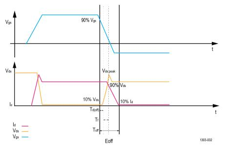
Figure 43: Waveform during turn off time
