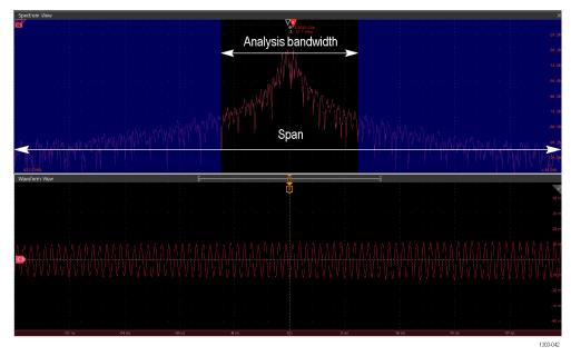
Figure 34: The image shows the analysis bandwidth for a given OBW measurement.
