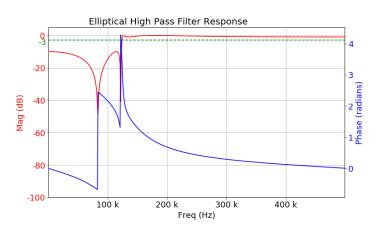
This filter is used in many RF and microwave applications where a very fast transition between the passband and stop-band frequencies is required.
