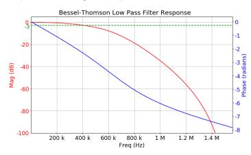
These filters are used in applications where a constant group delay is critical, such as in analog video signal processing.
