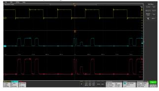
4. Double-tap a channel badge to open that channel's configuration menu to check or change settings. See *Configure channel and waveform settings* on page 96.
