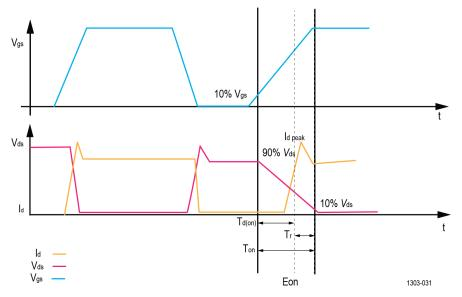
Figure 42: Waveform during turn on time
