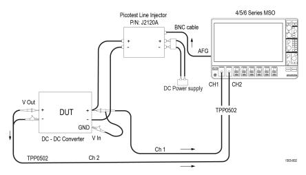
Figure 16: Connection diagram for PSRR measurement
