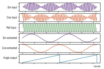
The mechanical measurements with Resolver takes three analog input waveforms, sin, cos, and ref. Ref is the excitation signal, where as sin and cos are output coil signals. Sin and cos signals are modulated with ref signal. Sin and cos envelopes have to be extracted before measuring various parameters with them. The envelope, which is the output of extraction, will be sin and cos signals, with an offset of 90 degrees in between them.
