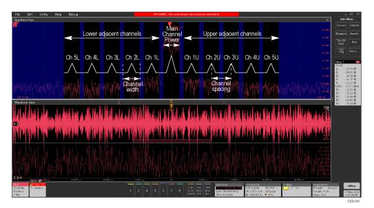
Figure 33: The image shows the channel width, channel spacing, and adjacent channels for a given ACPR measurement.
