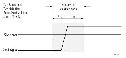
Setup/hold triggering uses the setup/hold violation zone to detect when data is unstable too near the time it is clocked. Each time trigger holdoff ends, the instrument monitors the data and clock sources. When a clock edge occurs, the instrument checks the data stream it is processing (from the data source) for transitions occurring within the setup/hold violation zone. If any occur, the instrument triggers with the trigger point located at the clock edge.
