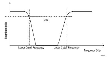
BSF filters are extensively used in Medical electronic systems.
