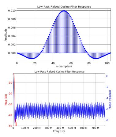
As impulse response starts, looking closer to a sinc response, the rate of magnitude transition increases rapidly to an extent where gain of output waveform start decreasing and also ripples in output waveform increases. It is advised to decrease the sample rate and symbols configuration in such situations. There will be a constant group delay in filtered output which can be removed by UDF "All Pass filter" if necessary.
