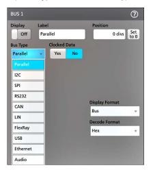
3. Use the fields and controls to select the bus signal sources, thresholds, other parameters, and the output format. The following image shows the settings for an Audio I2S serial bus.
