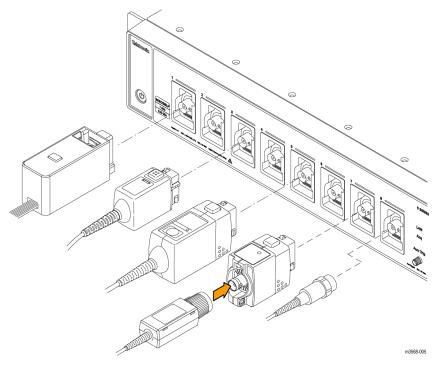
Figure 3: Connecting probes to the MSO58LP
