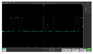
3. Continue tapping Inactive Channel buttons to add more channels (digital or analog). Channels are displayed from lowest-numbered channel at the top, to highest-numbered channel at the bottom of the view, regardless of the order they were added (in stacked mode).
