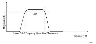
BPF is used in HSS (High Speed Serial) analysis for doing jitter measurements over a frequency range of interest. BPF can be used in Pre-amplification, Equalization and Control in Audio Systems applications.
