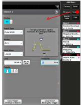
2. Use the configuration menu fields to set the search criteria in the same way that you would set for a trigger condition (select the **Search Type**, **Source**, and conditions on which to search).
