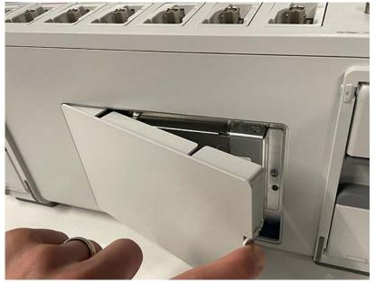
4. Slide the connector end of the SSD into the drive connector bracket. Push firmly to seat the drive in the connector.
