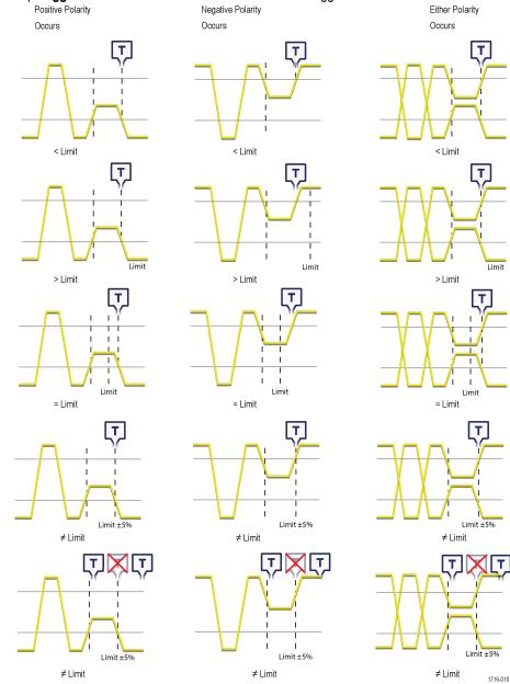
4. Tap Trigger When and select the condition on which to trigger.
