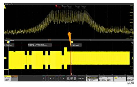
Using cursors in the Waveform View, the measured time from power-up to when the SS clock signal is stable was 4.847 seconds.
