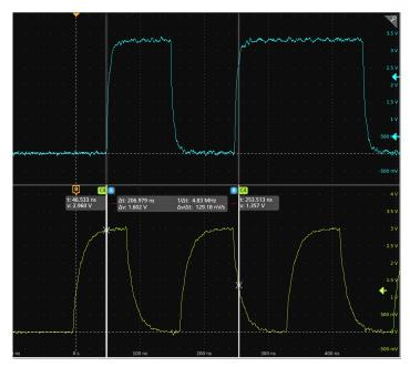
To further configure cursors, double-tap on either cursor line or the cursor readouts to open the Cursors configuration menu. For example, tap the Cursor type to select the cursors to display, such as Waveform, V Bars, H Bars, and V&H Bars. See Cursor configuration menu on page 424.
