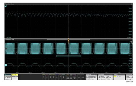
This trace can help characterize frequency modulation, frequency drift, and brief changes in frequency that might not be obvious in the spectrum trace.
