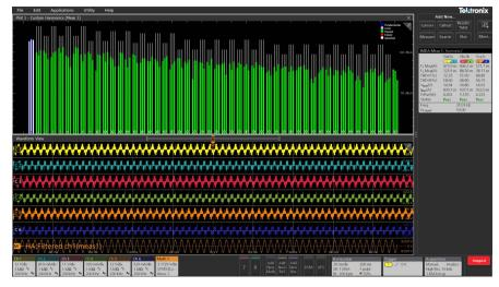
Figure 24: Harmonics with custom limits
