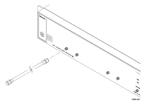
Figure 5: Connecting SMA cables to the LPD64
