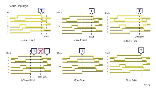
9. Tap Define Logic and set the logic condition that must occur with all specified signals to cause a trigger event.
