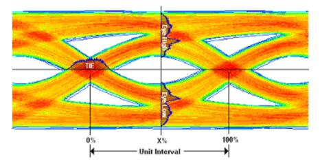
**Note:** This illustration shows how the measurement is made, and does not represent how the oscilloscope actually displays an eye diagram or histograms on an eye diagram plot.
