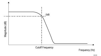
LPF are used to remove background and high frequency noise.
