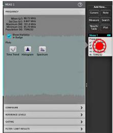
2. Tap a Plots button to add that plot for the measurement to the screen.
