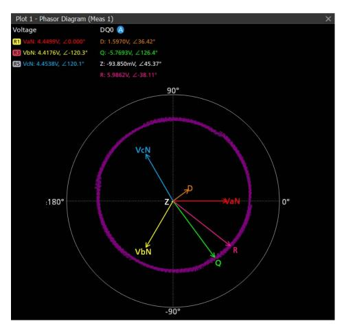
There are two angles, initial angle and incremental angle. The initial angle is where QEI Z index pulse starts and D-axis gets aligned at this position. This is not applicable in case of no Z index pulse.
