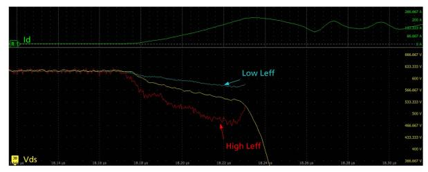
Figure 38: Vds modelled using low L<sub>eff</sub>(blue) and high L<sub>eff</sub>(red) to match zero skew acquired V<sub>ds</sub>(yellow) during turn on transient
