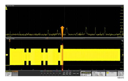
The Spectrum Time Bar position was slowly moved to the right until a valid SS clock signal was shown in the Spectrum view, as shown in the following image.
