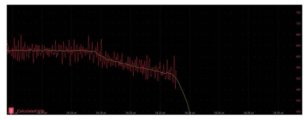
Figure 41: Noisy model of Vds using small differential order filter at turn on transient
