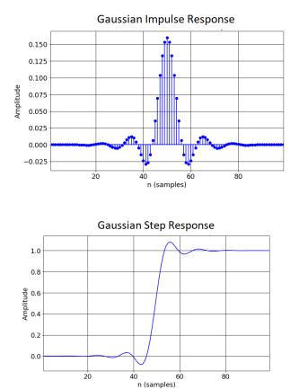
The standard deviation is a user input that defines the Gaussian window width.
