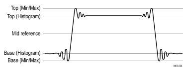
**Histogram Mean** uses histogram analysis to calculate the mean or average value using all values above and below the waveform midpoint. Top is set to the mean high value, and Base is set to the mean low value. This setting is best for examining eye patterns and optical signals.
