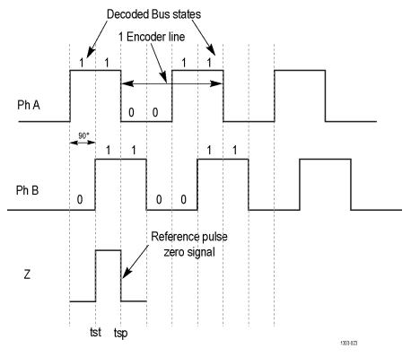
The tst start time of the Rise edge of the Phase A or B signal comes immediately after index Pulse Z rise edge. The tsp is stop time on next rise edge corresponding Phase. The Rise edge is taken after the index Pulse Z rise edge.
