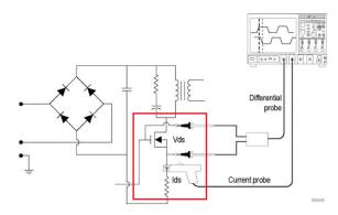
SMPS circuit diagram shows the points where switching loss can be measured. After full wave rectification, the current signal should pass through the harmonic standard and enters for DC conversation. MOSFIT plays an important role to meet the design of SMPS.
