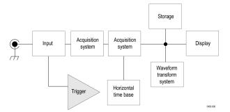
Trigger helps you to capture meaningful waveforms to display on screen. This instrument has simple edge triggers as well as a variety of advanced triggers.
