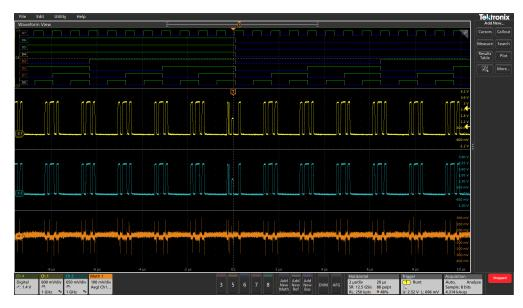
**Note:** Waveforms do not need to be displayed to be used for measurements, as long as the channel or waveform badge is on the **Settings** bar and is acquiring the signal to measure.
