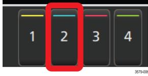
The selected channel is added to the Waveform View and a Channel badge is added to the Settings bar.
