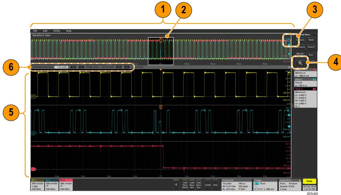
1. The **Zoom Overview** shows the entire waveform record. All waveforms are shown in Overlay mode in the Zoom Overview area.
