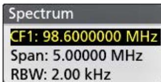
Tap the **Spectrum** badge to show the **Span** buttons to quickly increase or decrease the Spectrum trace span. Changing the span for one Spectrum trace changes the span for all traces.
