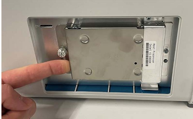
5. Push down on and tighten the thumb screw to attach the SSD to the chassis.
