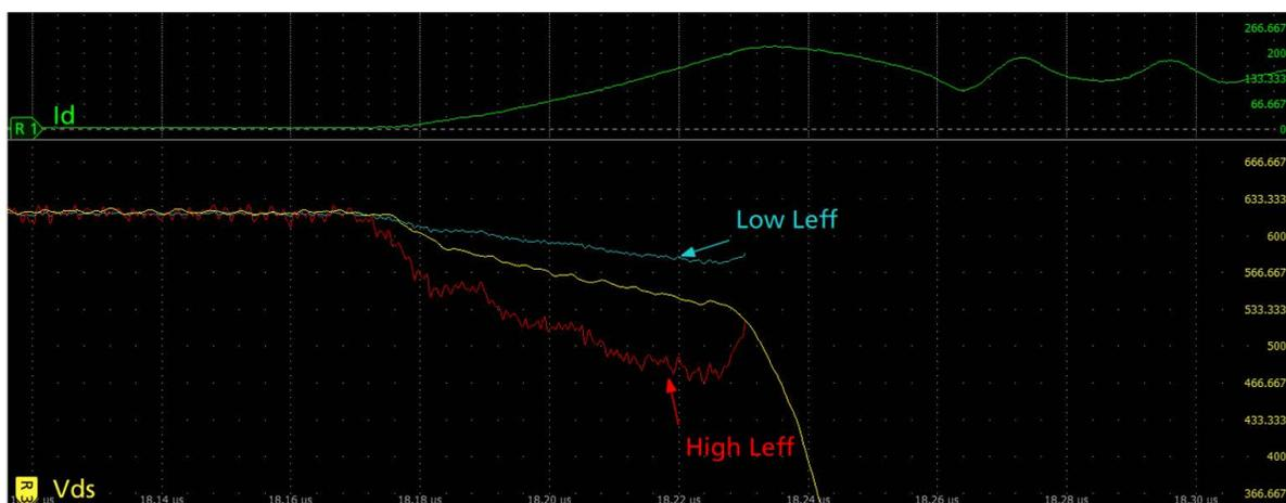
Figure 38:  $V_{ds}$  modelled using low  $L_{\text{eff}}$ (blue) and high  $L_{\text{eff}}$ (red) to match zero skew acquired  $V_{ds}$ (yellow) during turn on transient
