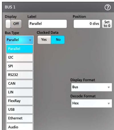
3. Use the fields and controls to select the bus signal sources, thresholds, other parameters, and the output format. The following image shows the settings for an Audio I2S serial bus.
