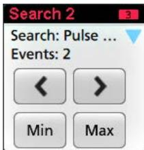
Some searches also provide **Min** and **Max** navigation buttons that open the Zoom mode and center the waveform in the display at the minimum or maximum value for that search event in the current acquisition.
