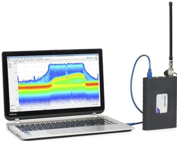
The RSA306 uses your PC and Tektronix SignalVu-PC™ RF Signal Analysis Software to provide real time spectrum analysis, streaming capture and deep signal analysis capabilities for signals from 9 kHz to 6.2 GHz, all in a low-cost, highly portable package that is ideal for field, factory, or academic use.
