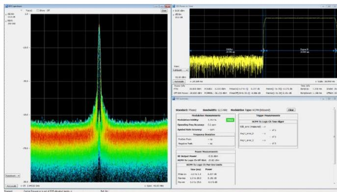
Sophisticated WLAN measurements are easy. On the displayed 802.11g signal, the spectrogram shows the initial pilot sequence followed by the main signal burst. The modulation is automatically detected as 64 QAM for the packet and displayed as a constellation. The data summary indicates an EVM of -33.24 dB RMS, and burst power is measured at 10.35 dBm. SignalVu-PC options are available for 802.11a/b/j/g/p, 802.11n and 802.11ac to 40 MHz bandwidth.
