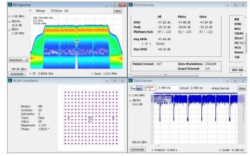
Analysis options for 802.11 standards are available. Here, an 802.11ac 80 MHz signal is analyzed, with displays of constellation, amplitude vs. time, summary of WLAN measurements, and the DPX spectrum of the analyzed signal. The density of the 'shoulders' of the WLAN signal are clearly seen in the DPX display, and a marker has been placed on the suppressed center carrier of the signal. An EVM of -47.65 dB and other signal measurements are seen in the summary panel
