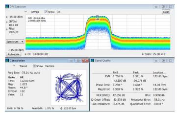
Multi-domain views provide a new level of insight into design or operational problems not possible with conventional analysis solutions. Here vector modulation quality and constellation (Opt. 21) are combined with the continuous monitoring of the DPX<sup>®</sup> spectrum display.
