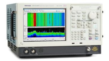
The RSA6000 Series gives you the functionality of a high-performance spectrum analyzer, wideband vector signal analyzer, and the unique trigger-capture-analyze capability of a real-time spectrum analyzer - all in a single package. A typical 20 dBm TOI and -151 dBm/Hz DANL at 2 GHz gives you the dynamic range you expect for challenging spectrum analysis measurements.
