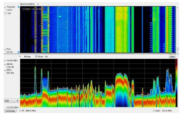
DPX Spectrograms provide gap-free spectral monitoring for up to days at a time. 60,000 traces can be recorded and reviewed, with resolution per line adjustable from  $110 \ \mu s$  to  $6400 \ s$ .
