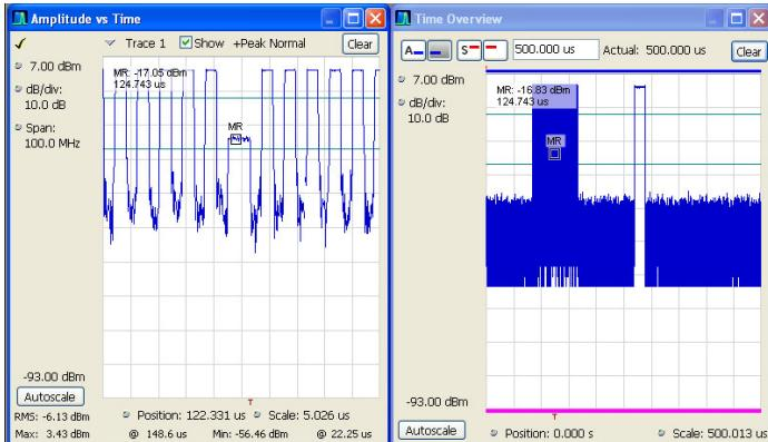
Advanced Triggers and Swept DPX (Opt. 200) combines the revolutionary DPX Density Trigger with the ability to trigger on runt pulses and apply time qualification to any trigger. The runt trigger seen here can be used to track down nonconforming pulses in a pulse train, greatly reducing time to insight. Time qualification can be used to separate ranging pulses from higher resolution pulses in a radar signal, or trigger only on signals that remain on longer than a specified time.
