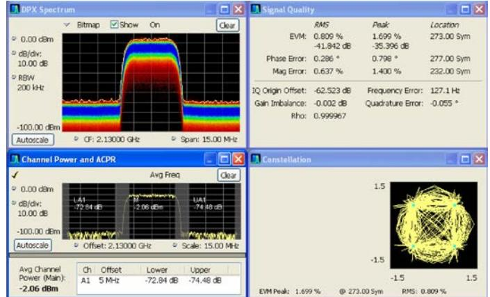
Time-correlated, multidomain views provide a new level of insight into design or operational problems not possible with conventional analysis solutions. Here, ACLR and Vector Modulation Quality (Opt. 21) are performed on a single acquisition, combined with the continuous monitoring of the DPX® spectrum display.
