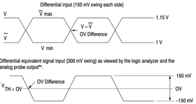
\* Note: For differential inputs, the module threshold should be set to OV (assuming no common mode error).
